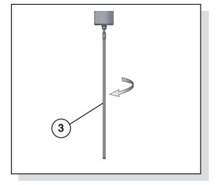
Dip the internal tube in hot water and Pulicaf detergent for 30 minutes (picture below). In order to remove any milk incrustations, clean the internal part of the sheath by means of the appropriate pipe-cleaner (4) you will find in the machine outfit (picture below).
